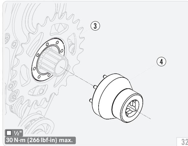
**NOTICE** Incorrect removal may damage the chain ring by distorting it.
