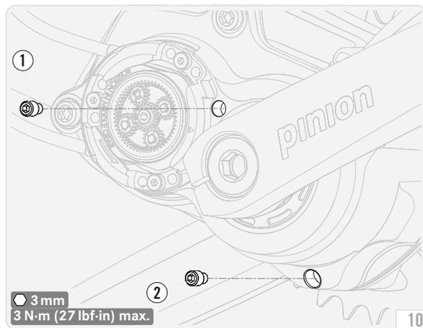
→ Place the bicycle or secure it in the repair stand so the drain opening is at the lowest point of your Pinion gearbox.
