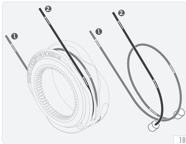
**NOTICE** Correctly wound up shifting cables will not cross over one another at any point!
