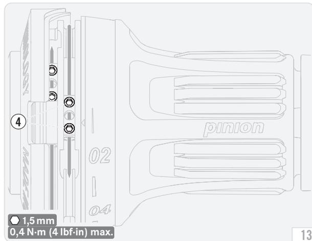
**① INFO** The clamp screws are easily accessible at rotary shifter positions **01 and 12** or **01 and 09** or **01 and 06** depending on the type of your Pinion gearbox.
